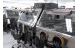
▲The anaerobic experimental system* that creates anaerobic and hypoxic conditions
