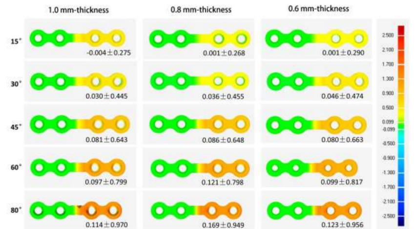
Figure 3 The registration colored map and the mean ( $\pm$  virtual deviation) values of displacement deviations of the point cloud.
