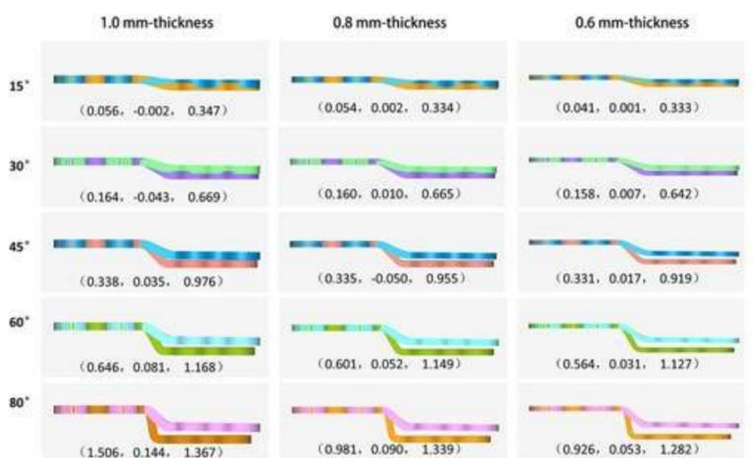
Figure 5 The lateral views of the registered models and the values of displacement deviations of the right end in the 3-dimensional coordinate system (x, y, z).
