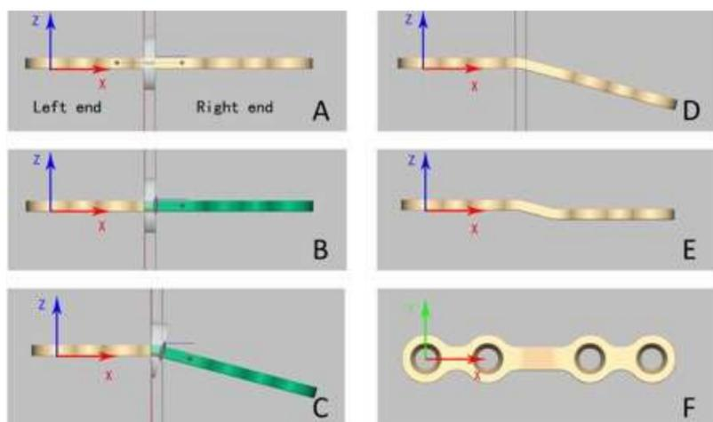
Figure 1 The virtual bending simulation. The simulation of virtual bending process of titanium miniplate in preoperative virtual surgical.
