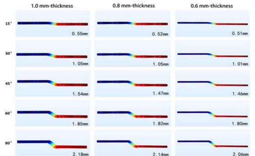
Figure 4 The lateral views of pre-bent titanium miniplate models and the final displacements of the right end in Z axis in the manual bending simulation.
