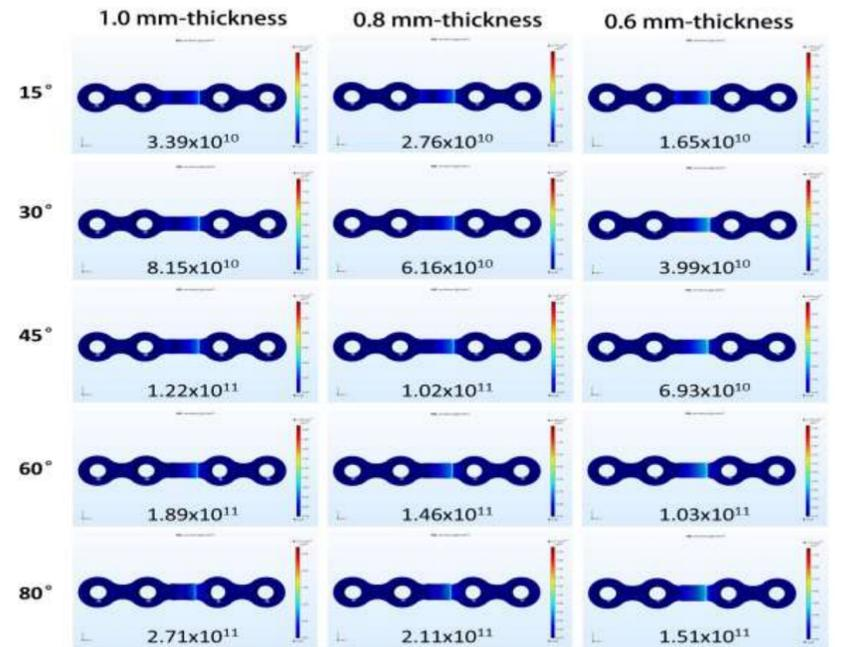
Figure 2 The stress distribution of the pre-bent titanium miniplate models and the value of maximum stress in the manual bending simulation.
