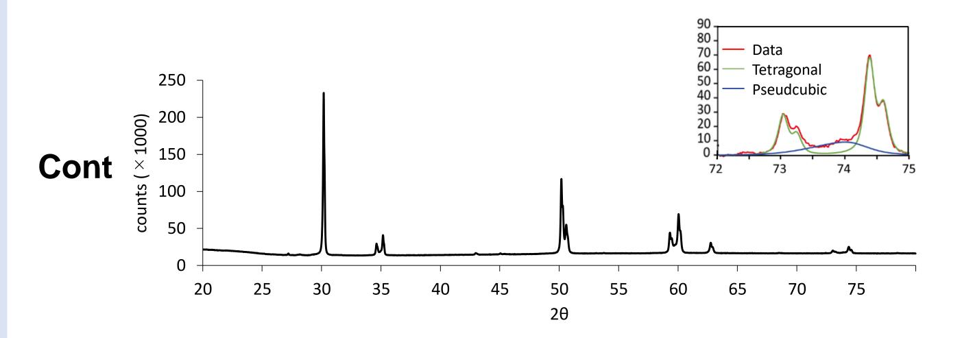
Rietveld analysis revealed that conventional zirconia was composed of **79% tetragonal phase** and **21% pseudocubic phase**.
