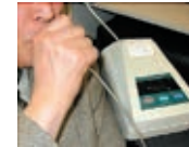
◀ Portable measuring system of oral malodor
