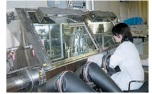
▲ Anaerobic chamber, simulating anaerobic conditions in oral biofilm.
