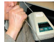
◀ Portable measuring system of oral malodor
