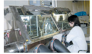
Anaerobic chamber, simulating anaerobic conditions in oral biofilm.
