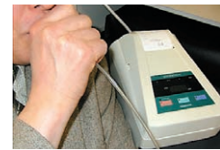
Portable measuring system of oral malodor
