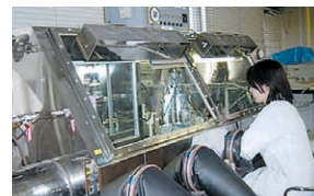
Anaerobic chamber, simulating anarobic conditions in oral biofilm.
