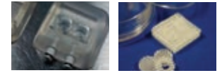
▲Development of the culture device to load a mechanical stress on osteoblasts and chondrocytes. Analysis of stem cell differentiation process into osteoblasts and chondrocytes using the micro-nano manipulation technology.
